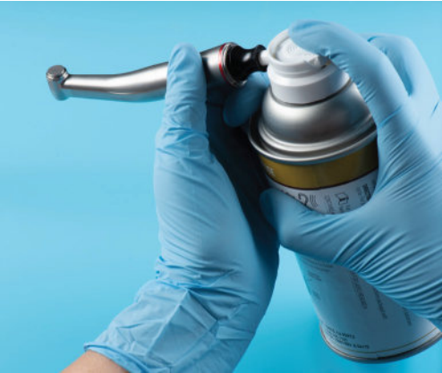
Figure 5: Photo of lube can with nozzle inserted into back of a contra-angle
