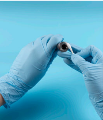
Figure 6a and 6b: Photo of fiber optics being cleaned at both ends with cotton swab.
