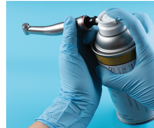
Figure 5: Photo of lube can with nozzle inserted into back of 1:5 contra-angle
