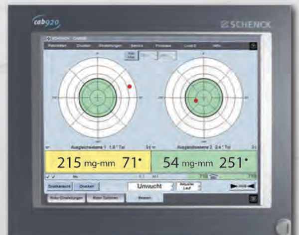
A dynamic balancing machine displays rotor imbalance
